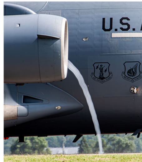
Figure 1. A ground vortex's low-pressure core visualized by condensed water vapor on a Boeing C-17 Globemaster III during reverse thrust (Lindsay, 2023).
