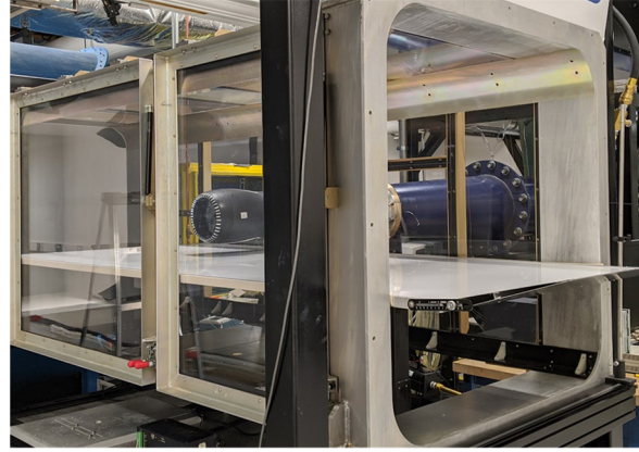
Figure 1. The crosswind wind tunnel test section showing the installed axisymmetric inlet and the moveable ground plane.
